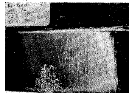
Fig. 55. Bright nickel plating bath (28) Contaminated with large amount of zinc 2.0 amp 55°C pH 5.5 5.7 v 10 min
